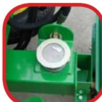
In line hydraulic filter with guard on cover
