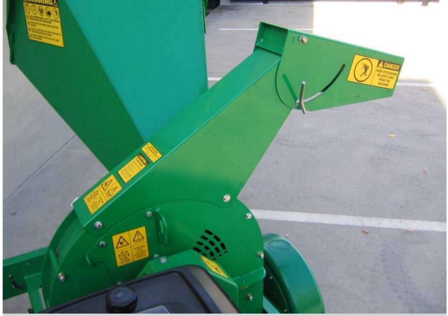
Fixed Discharge Chute – Reduces Clogging
