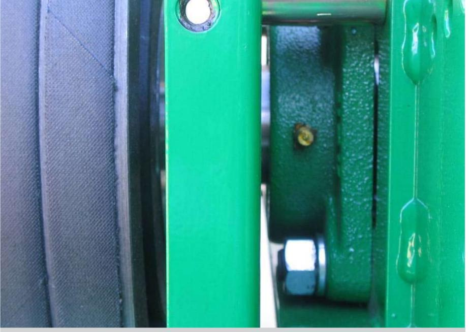
Rear Rotor Bearing Grease Fitting
