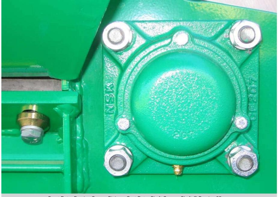
Front Rotor Bearing Grease Fitting – Cast Rotor Shaft Cover – Shaft @ Bearing 35mm
