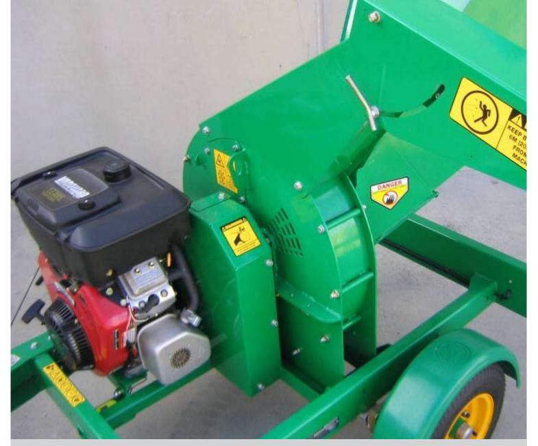
Fixed Discharge Chute with Adjustable Deflector
