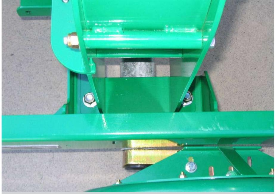
Laser Cut, CNC Folded, Sandblasted & Powder Coated Chassis
