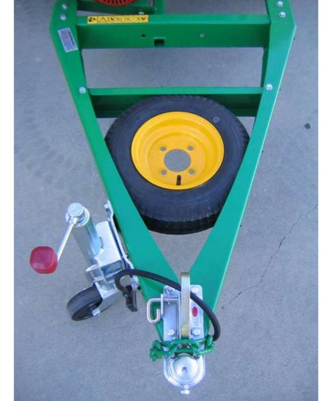
Spare Tyre Assembly Jockey Wheel 50mm Coupling 7-Pin Flat Connector
