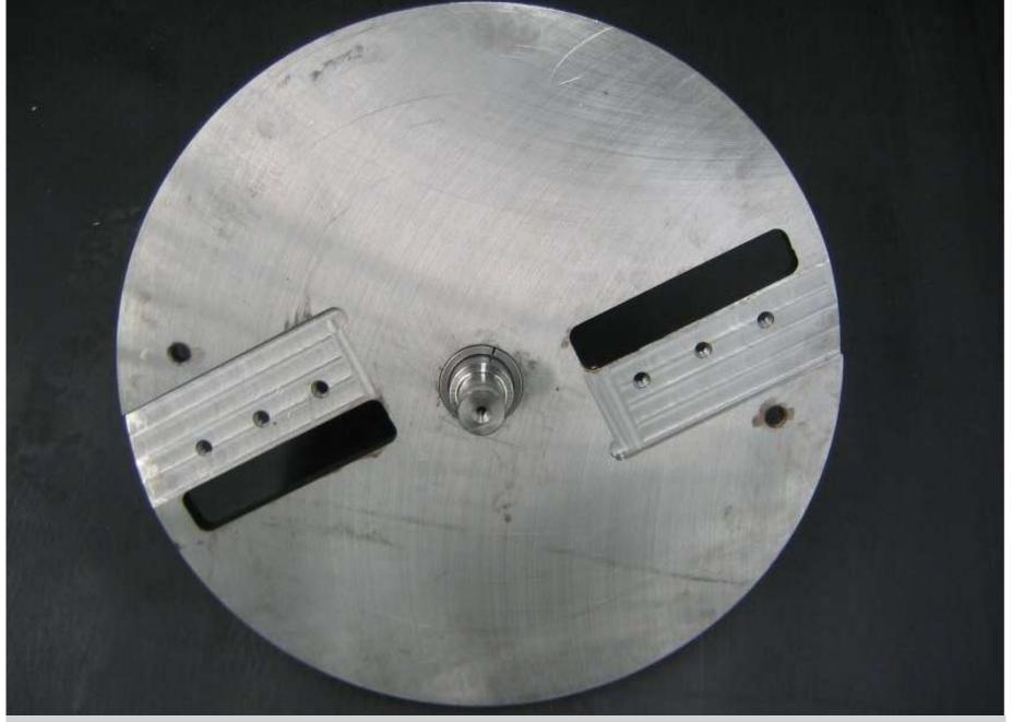
Front of Chipper Disc – 578mm (22.75") Diameter – 50mm (1.97") Shaft at Hub Centre
