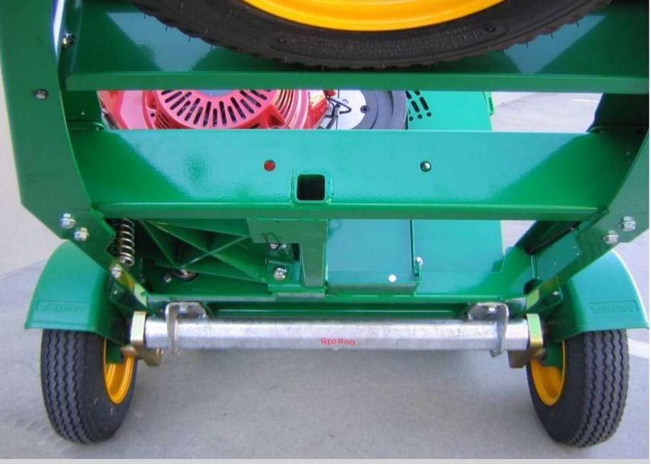
Red Roo Flexride<sup>™</sup> Independent Rubber Torsion Axle – Galvanized
