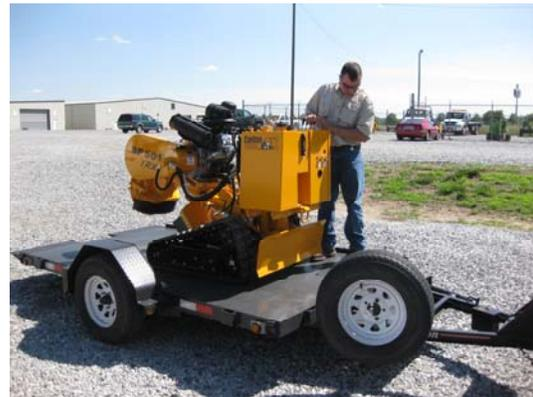
The model SP5014TRX can be loaded into a pick-up truck, but requires increased safety precautions against tipping. Tie-downs, a sturdy and stable loading ramp and extra caution are required.
