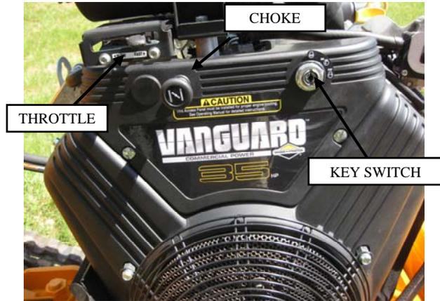
**DO NOT OPERATE THE ENGINE AT AN ANGLE GREATER THAN 25° OR SEVERE ENGINE DAMAGE WILL OCCUR. PROPER ENGINE OIL LEVEL MUST BE MAINTAINED TO ACHIEVE MAXIMUM ANGLE OF OPERATION OF 25°. (See Engine Owner's Manual for proper oil level.)**
