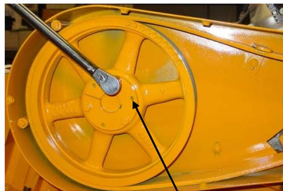
AFTER REMOVING BOLTS. SCREW BOLTS INTO THE THREADED HOLES TO PUSH THE BUSHING OUT OF THE PULLEY
