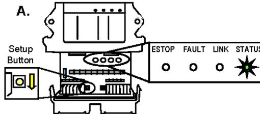
**NOTE 1:** The Receiver will hold up to 4 Transmitter ID's. When the 5th Transmitter ID is downloaded, it's ID will replace the ID of the least recently used transmitter (i.e. The receiver will retain the ID's of the three transmitters that have been most recently linked).
