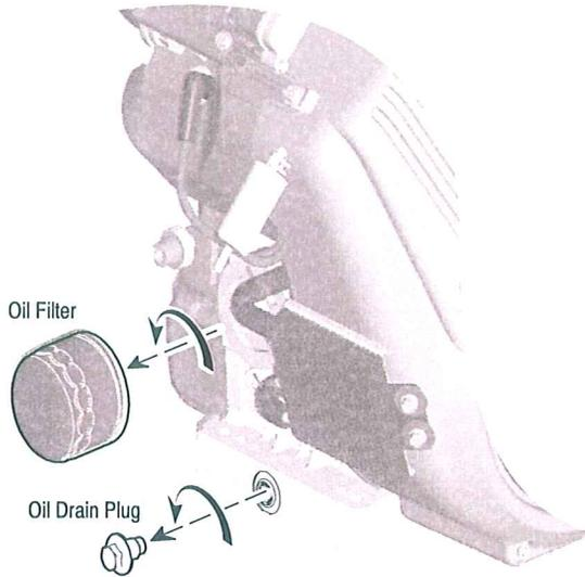
1. With engine OFF but still warm, remove oil drain plug and drain oil into appropriate receptacle. Reinstall drain plug.
