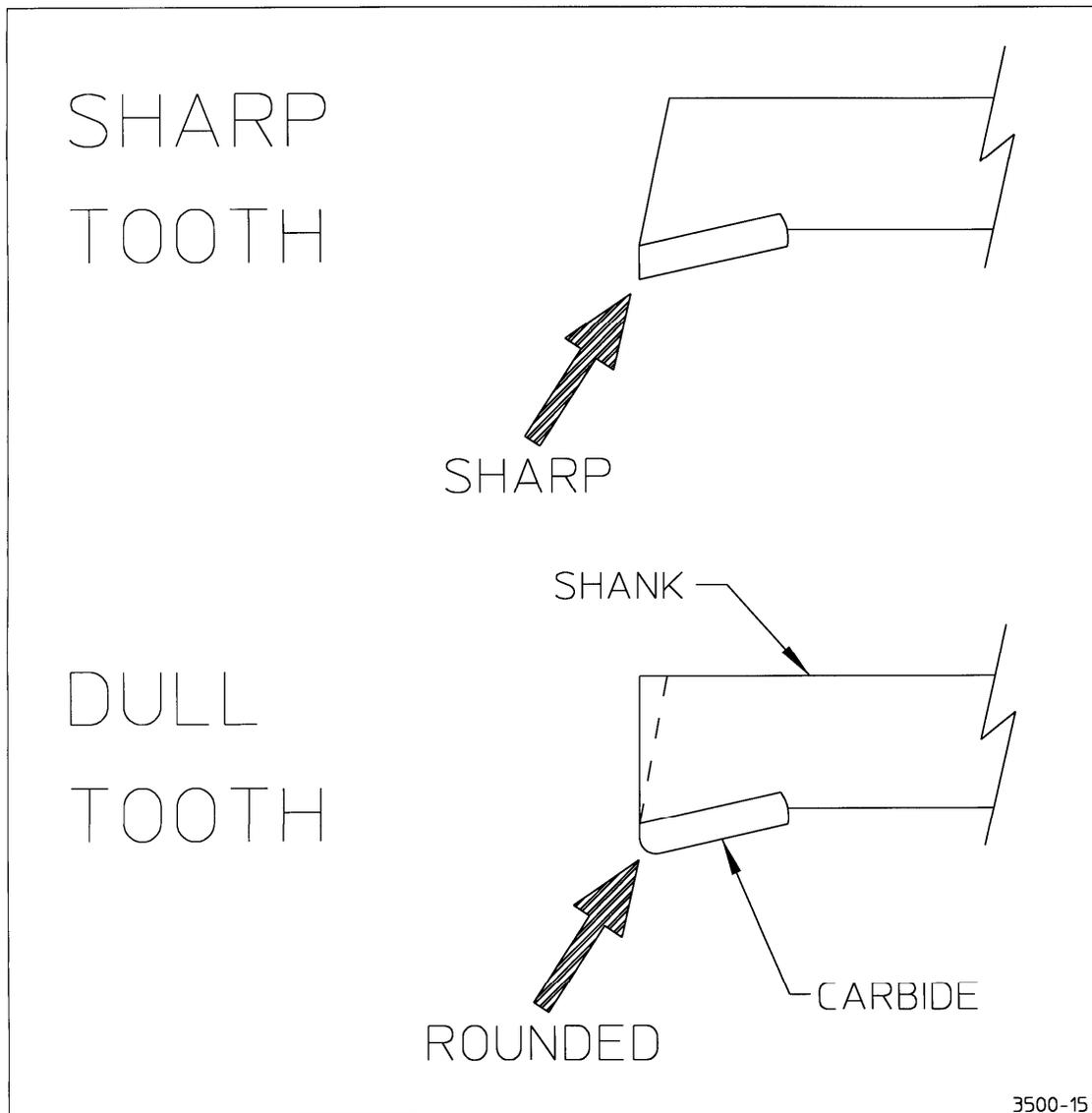
Begin by chamfering shank back past edge of carbide. You do this because if it is not back far enough the shank will hit the stump and not the carbide, thus causing a lot of vibration. Once the shank is angled far enough back, then begin sharpening carbide.
