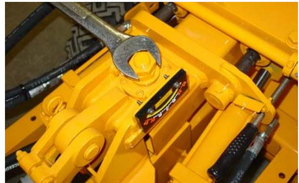
If the main pivot bearings need replacing, you will have to remove the top pin and slide the main pivot out and install the new bearings. **See Upper Pivot Assembly for breakdown.**
