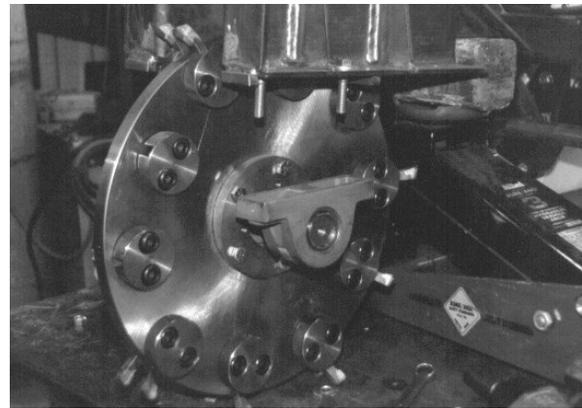
NOTE: To make shaft installation easier, place shaft in a freezer for approximately one hour or overnight if possible. This will shrink the shaft and make installation into the new bearings much easier.
