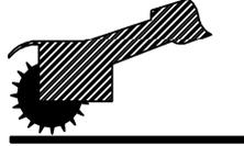
This machine may tip over sideways if operated on non level surface.
