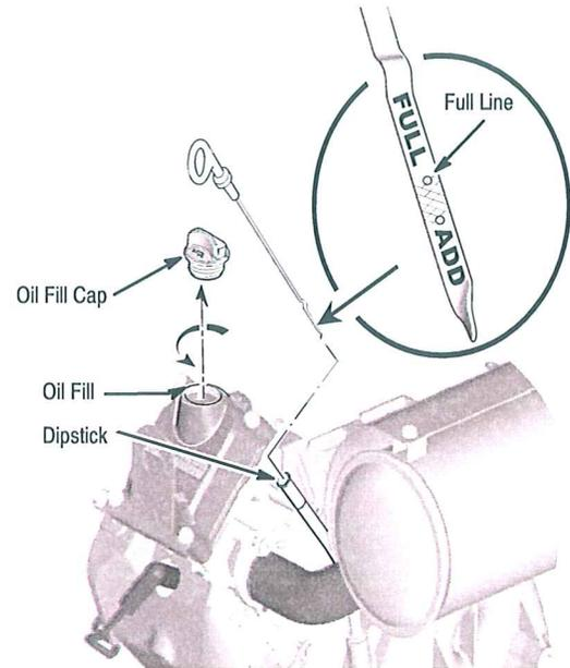
1. Place engine level and clean around oil filler plug.
