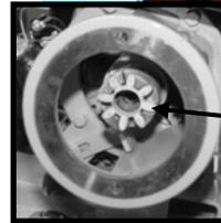
REPLACE THE RUBBER INSERT WHEN REATTACHING THE PUMP
