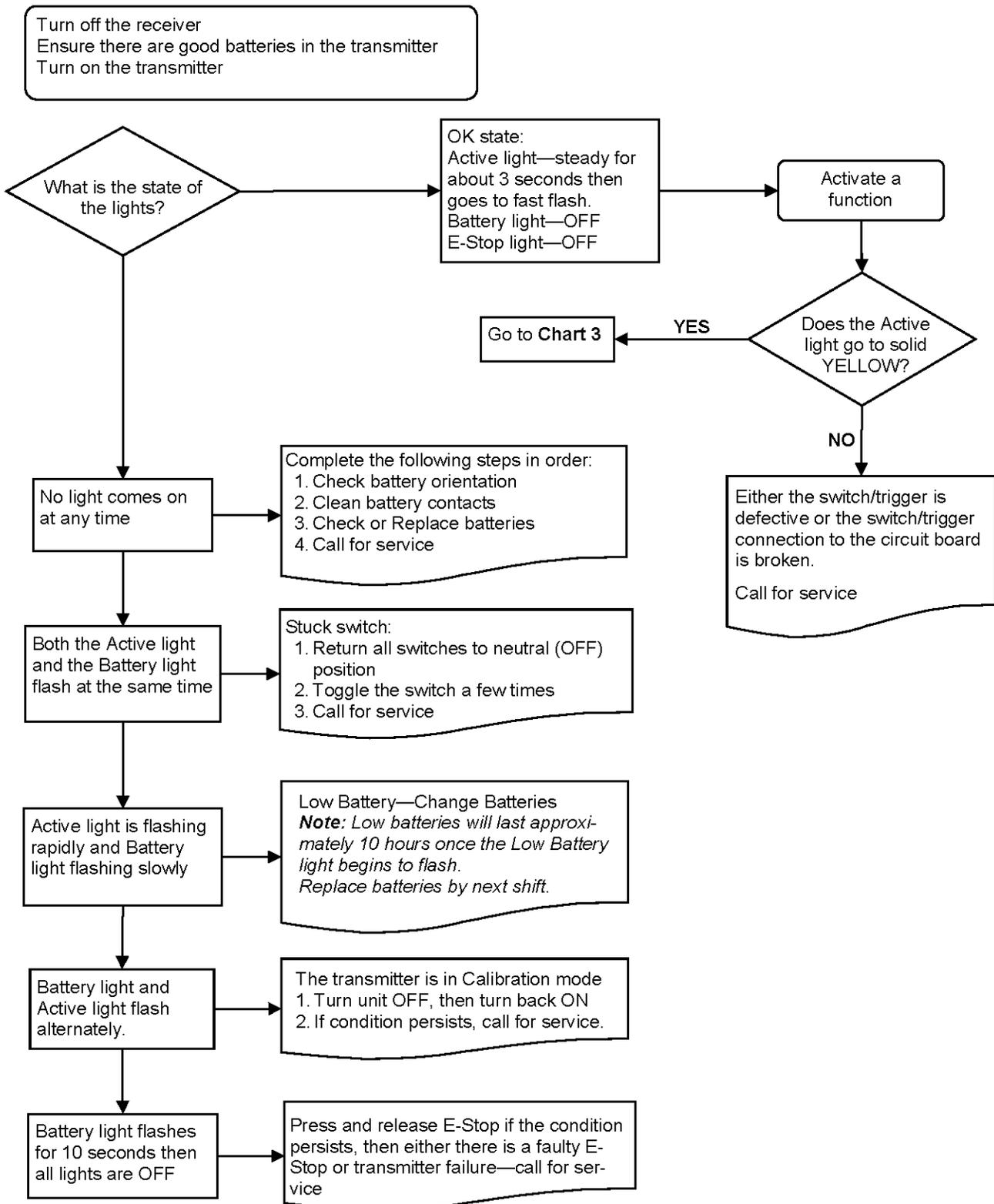
Testing the Transmitter / Receiver Communication
