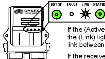
If the (Active) light on the transmitter is flashing and the (Link) light on the receiver is flashing GREEN, a link between the two exists.
