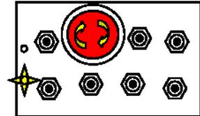
If the transmitter's (Active) light does not flash, check the battery orientation.
