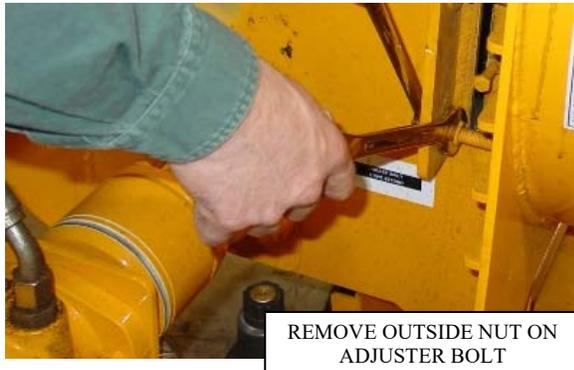
REMOVE OUTSIDE NUT ON ADJUSTER BOLT
