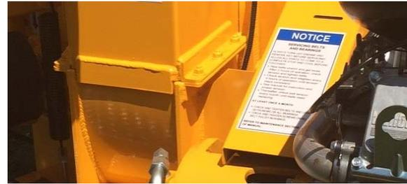
**DANGER:** Do not open the cutter disk hood until the cutter disk has come to a complete stop. Do not perform service on the cutter disk or knives without installing the disk lock pin.
