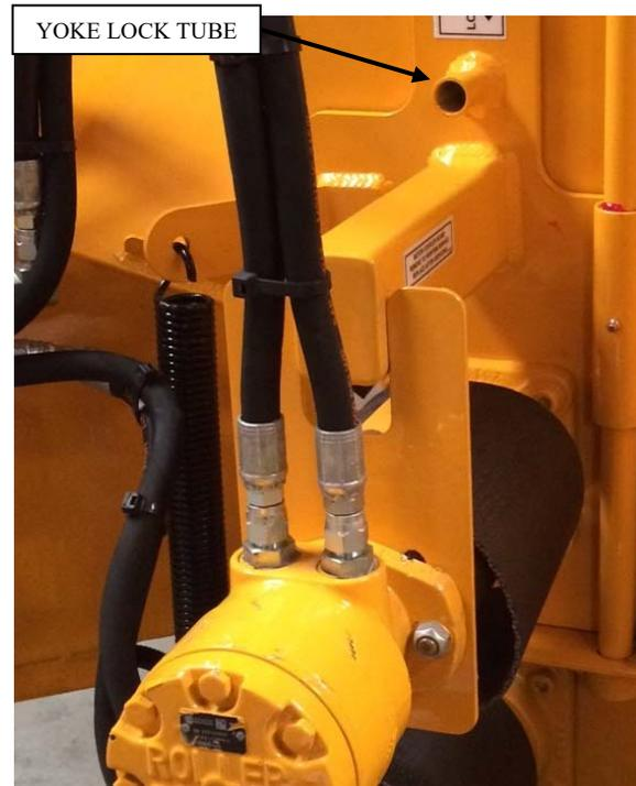
**When working with the feed wheel, the yoke lock pin must be inserted in the yoke lock tube after the feed wheel has been raised.**
