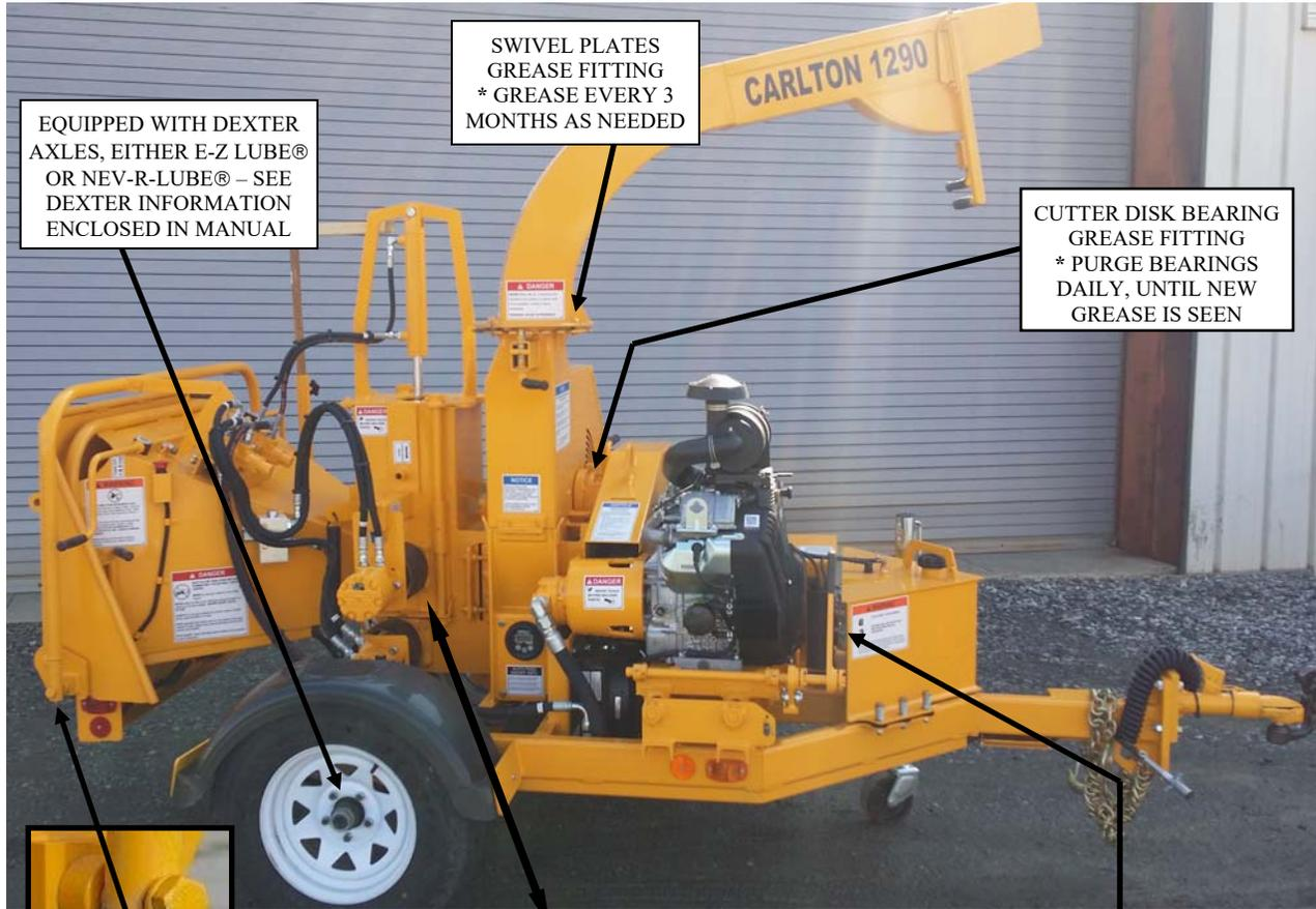
EQUIPPED WITH DEXTER AXLES, EITHER E-Z LUBE® OR NEV-R-LUBE® – SEE DEXTER INFORMATION ENCLOSED IN MANUAL
