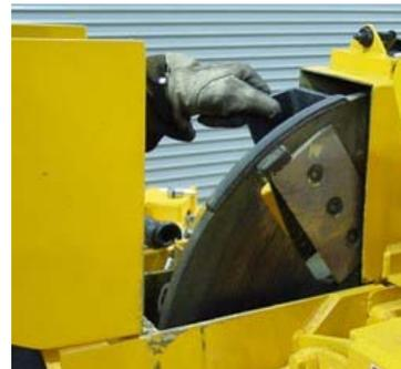
ROTATE CUTTER DISK TO CHECK FOR BINDING
