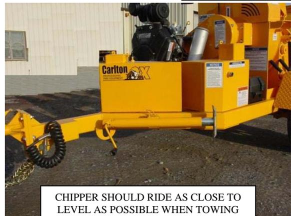
CHIPPER SHOULD RIDE AS CLOSE TO LEVEL AS POSSIBLE WHEN TOWING
