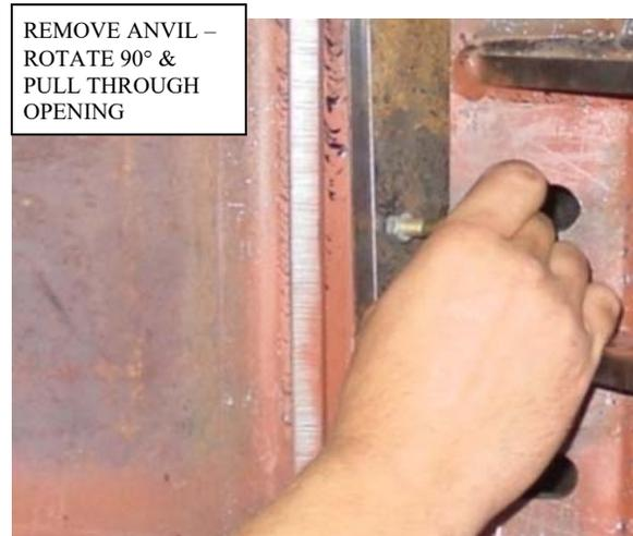
REMOVE ANVIL – ROTATE 90° & PULL THROUGH OPENING
