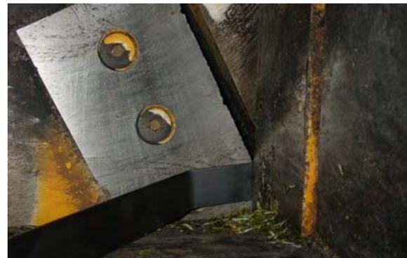
**THE CUTTER DISK HOOD IS ONE OF THE MOST IMPORTANT PIECES OF SAFETY EQUIPMENT ON THIS CHIPPER. MAKE SURE IT IS KEPT IN GOOD WORKING CONDITION.**
