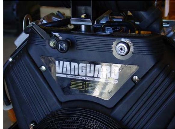
**DO NOT OPERATE THE ENGINE AT AN ANGLE GREATER THAN 25° OR SEVERE ENGINE DAMAGE WILL OCCUR. PROPER ENGINE OIL LEVEL MUST BE MAINTAINED TO ACHIEVE MAXIMUM ANGLE OF OPERATION OF 25°. (See Engine Owner's Manual for proper oil level.)**
