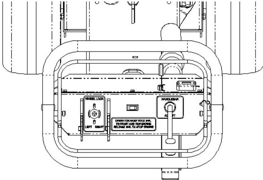
5. **ENGINE START:** Both Vanguard and Honda options are equipped with manual pull starts. The engine bail switch must be held down to allow the engine to start and run. If the bail is released, the engine will shut down. After the engine is running and warmed up, increase the engine speed fully to engage the centrifugal clutch and grinder wheel.
