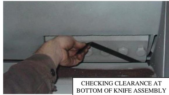
CHECKING CLEARANCE AT BOTTOM OF KNIFE ASSEMBLY
