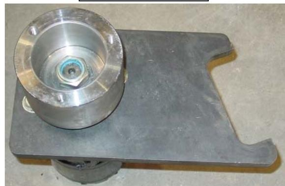
STRIKE THE COUPLING WITH RUBBER Mallet TO SEAT
