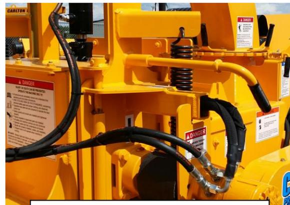
UPPER FEED WHEEL MUST BE RAISED, PINNED, AND BLOCKED
