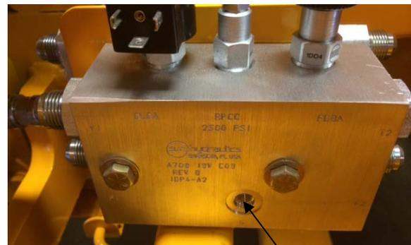
REMOVE PLUG AND INSTALL PRESSURE GAUGE
