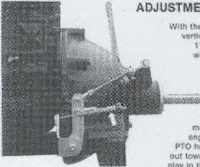
To adjust clutch linkage, loosen the two 5/8" hex nuts as shown in the picture by arrow. Check to make sure the PTO turns freely in the disengaged (handle horizontal) position. If the PTO has resistance to turning, adjust the nuts out toward the clutch fork. Check again for free play in the handle vertical position. After adjustments are made, lock the two 5/8" hex nuts together.
