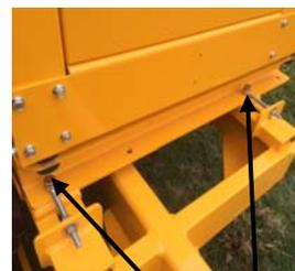
ENGINE SLIDE BOLTS - 2 AT FRONT OF ENGINE
