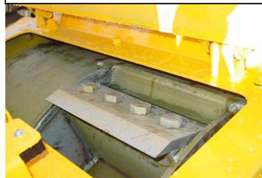
**DANGER: Do not open the cutter drum door until the cutter drum has come to a complete stop. Do not perform service on the cutter drum or knives without installing the drum lock pin.**
