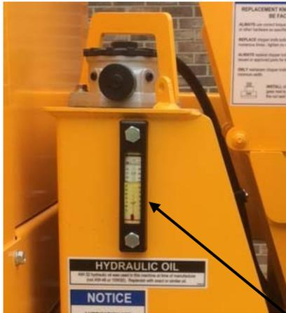
HYDRAULIC OIL SHOULD BE VISIBLE IN THE LEVEL/TEMP GAUGE, MAKE SURE THE OIL IS BETWEEN THE TOP BLACK LINE AND THE BOTTOM RED LINE (SEE SERVICING HYDRAULICS SECTION).
