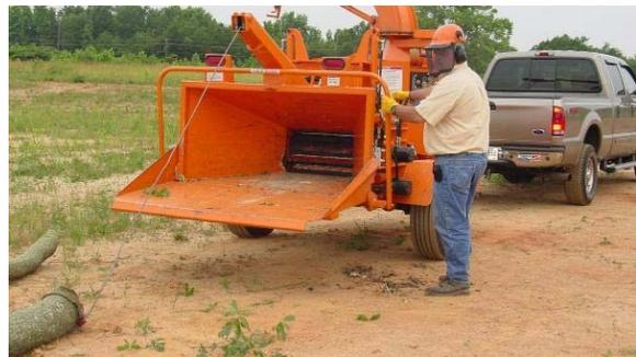
9. When the tree is in the infeed chute, remove the winch rope. Rotate the winch selector valve back to the left (clockwise) and follow the standard operating procedures for chipping the material.
