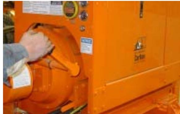
**CAUTION: Chipper disk will continue to spin even though it is disengaged!**
