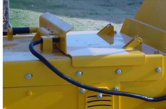
**THE CUTTER DRUM DOOR IS ONE OF THE MOST IMPORTANT PIECES OF SAFETY EQUIPMENT ON THIS CHIPPER. MAKE SURE IT IS KEPT IN GOOD WORKING CONDITION.**
