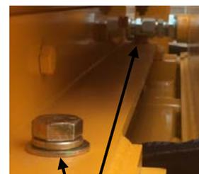
ENGINE SLIDE BOLTS - 2 AT BACK OF ENGINE
