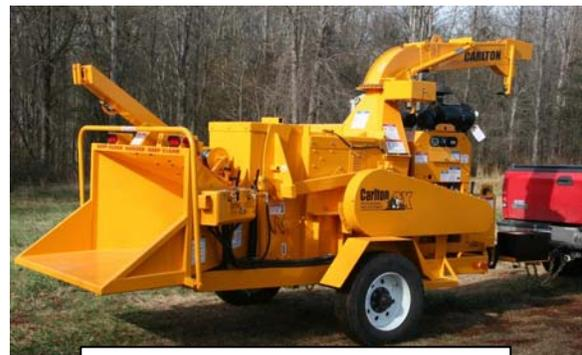
CHIPPER SHOULD RIDE AS CLOSE TO LEVEL AS POSSIBLE WHEN TOWING
