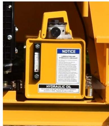
Check hydraulic oil level daily. This Carlton chipper is equipped with a gauge that shows the level of oil and the temperature of the oil. When filling the tank with oil, the window of the gauge will also fill with oil as the level gets higher in the tank. Never fill the oil tank above the BLACK line at the top of the gauge. Do not run the machine with the oil level below the RED line at the bottom of the gauge.
