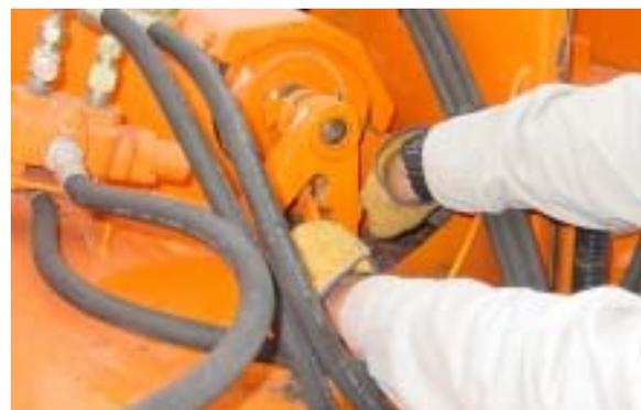
3. Pull the winch rope to the tree. Always wear leather gloves when handling winch rope. Broken wires will cause injuries.
