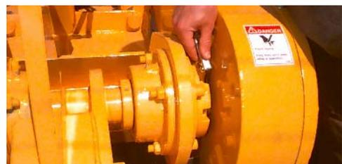
Always clean tip of grease gun fitting and grease fitting on machine before attaching hose to prevent dirt from being forced into machine parts.
