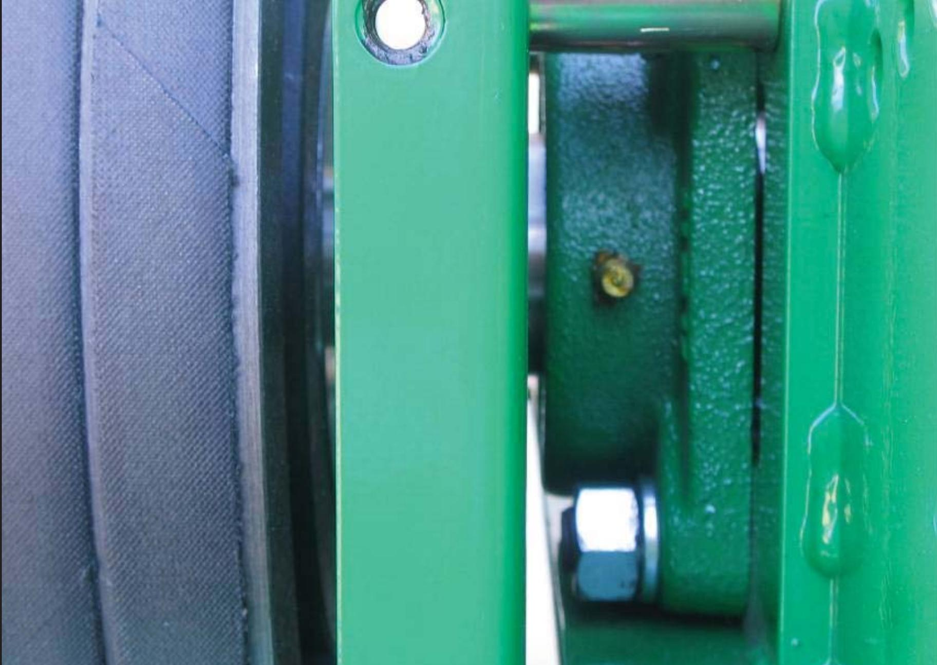
Rear Rotor Bearing Grease Fitting
