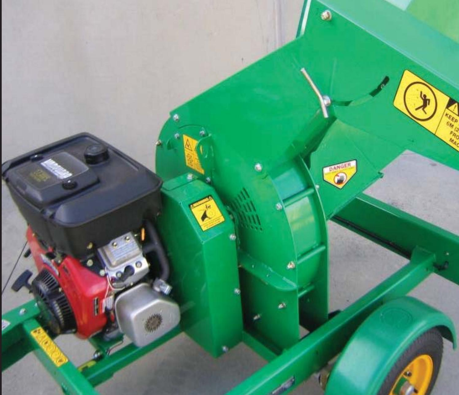
Side Discharge Chute with Adjustable Deflector
