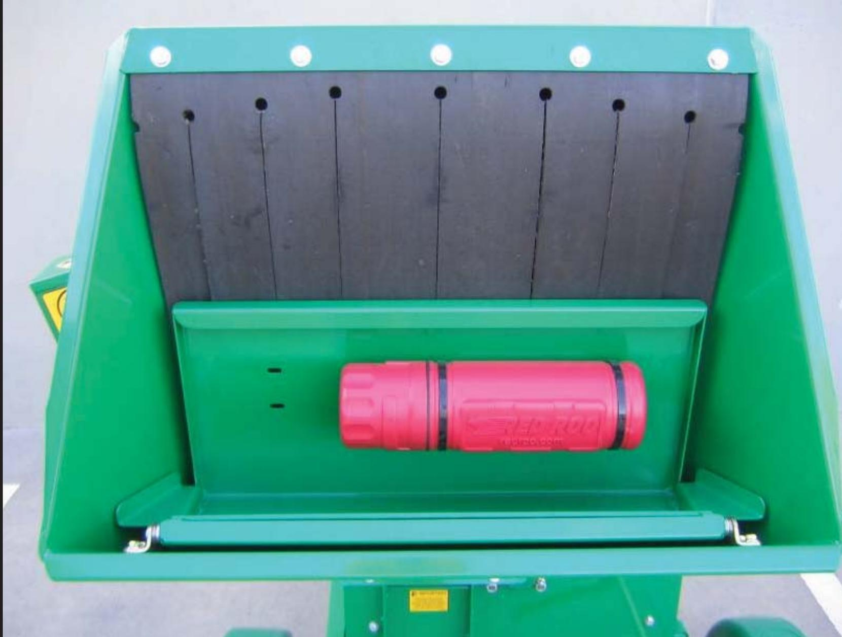
Guard with Operator Instruction/Tool Holder Infeed Chute
