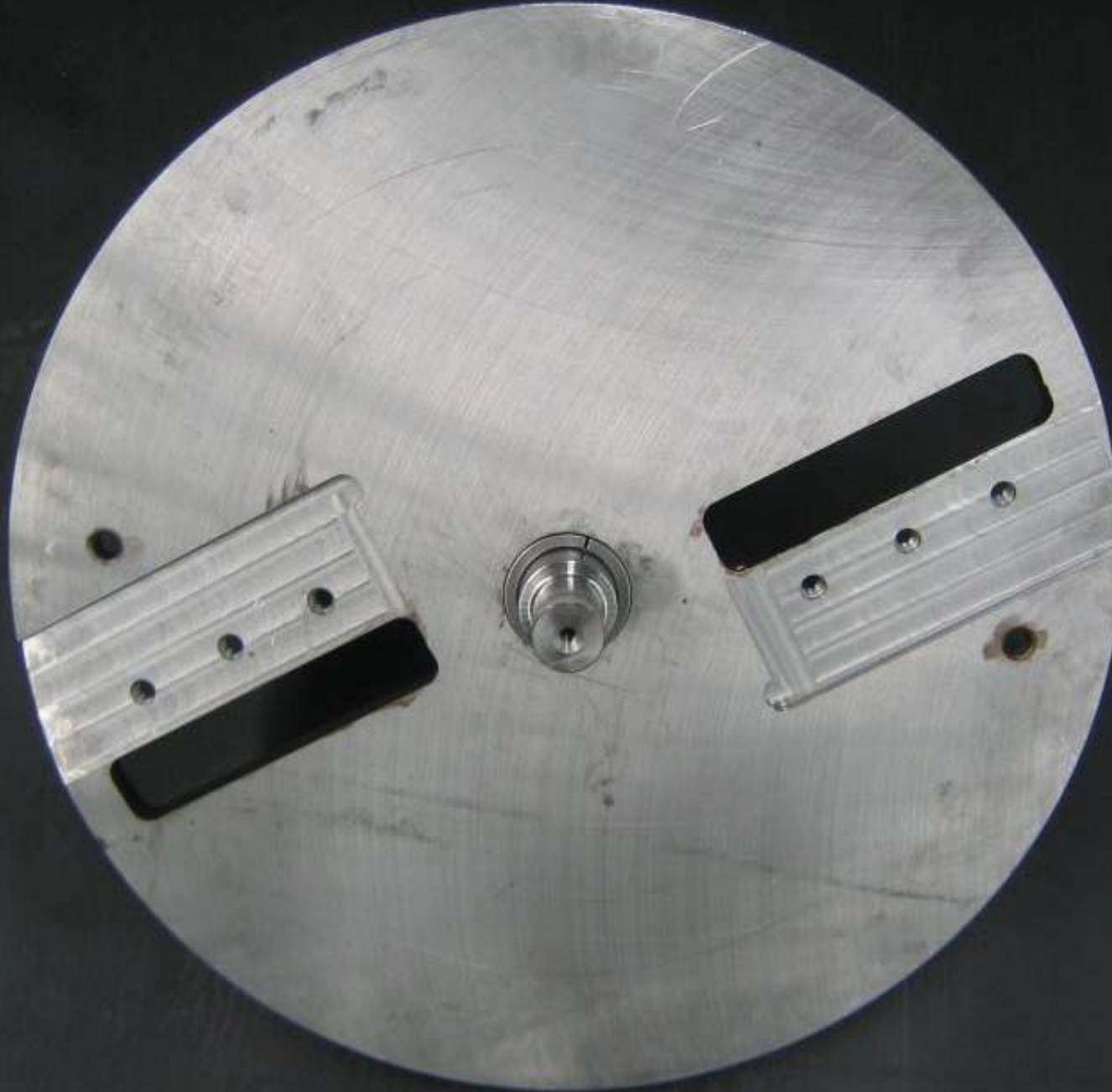
Front of Chipper Disc – 578mm (22.75") Diameter – 50mm (1.97") Shaft at Hub Centre
