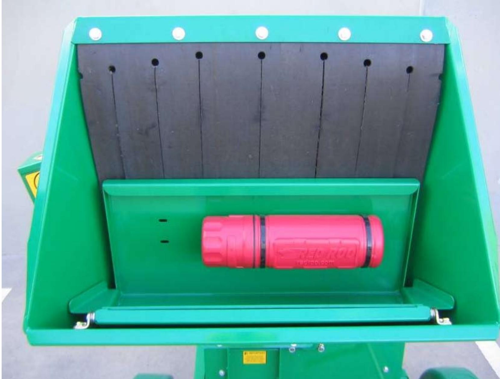
C80 Infeed Height – 1170mm / C100 Infeed Height – 1200mm
