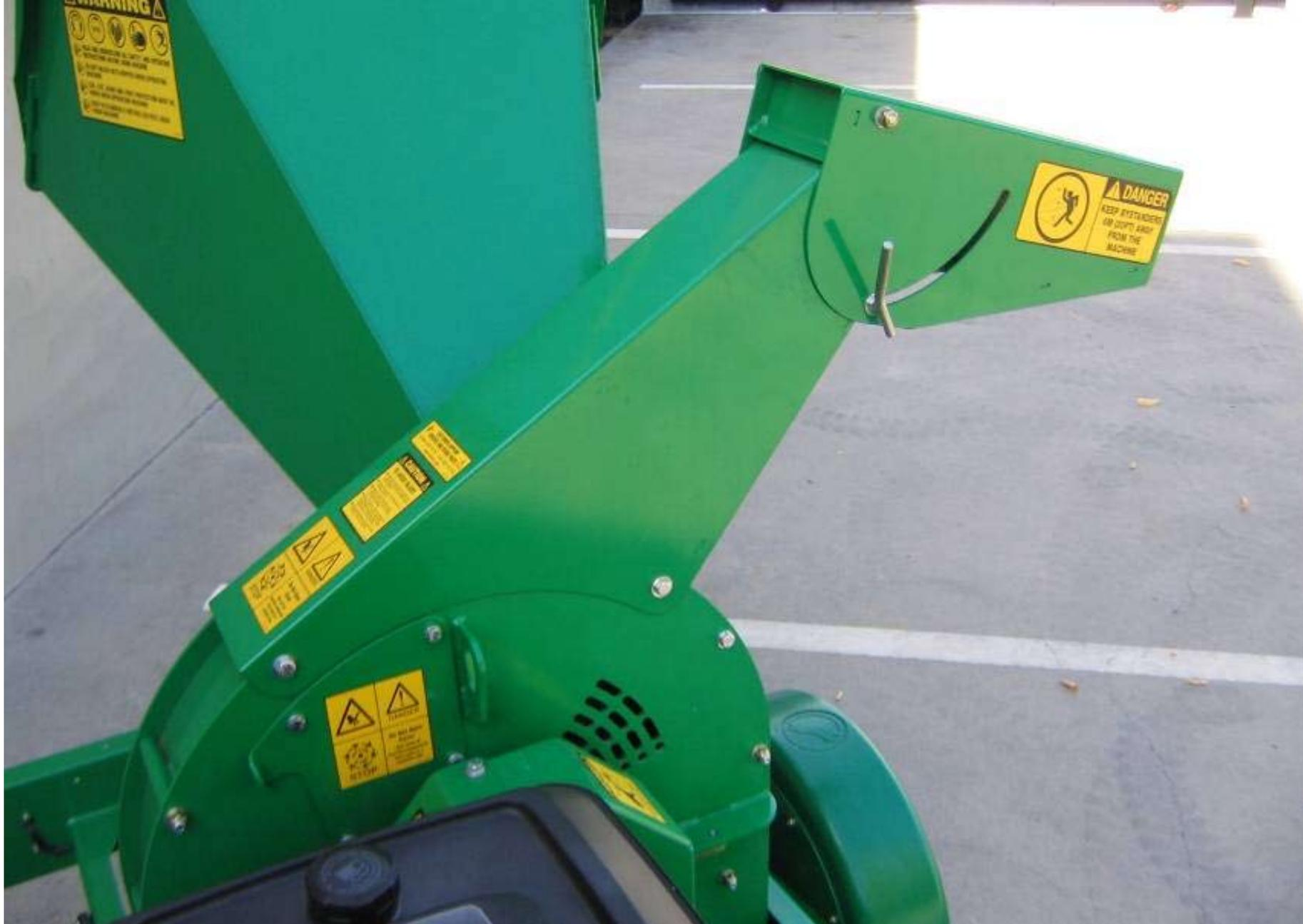
Fixed Discharge Chute – Reduces Clogging
