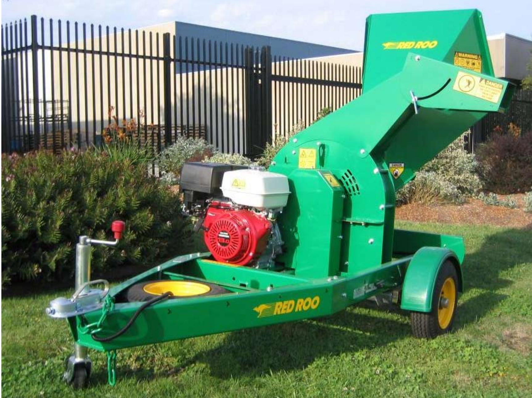
Red Rooster C80 Chipper with 13hp Honda GX390 Engine
