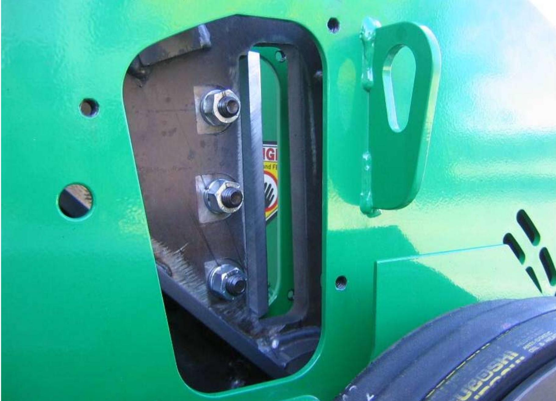
Blade Access with Disc Locking Pin In Use
