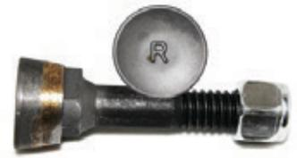
Cutting teeth may be sharpened by grinding. Initial sharpening should be performed using a silicon carbide (green) wheel. The best results will be achieved by finish grinding using a diamond grinding wheel.
