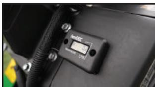
ENGINE HOUR METER/TACHOMETER
