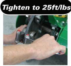
**BEFORE YOU REPLACE ANY CUTTERS YOU MUST TURN THE ENGINE OFF AND WAIT FOR ALL MOVING PARTS TO STOP. MAKE SURE ALL OF THE CUTTERS ARE SHARP AND WELL MAINTAINED AT ALL TIMES.**
