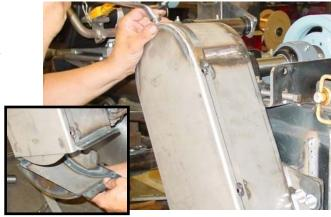
Loosen Poly Chain® belt by moving
