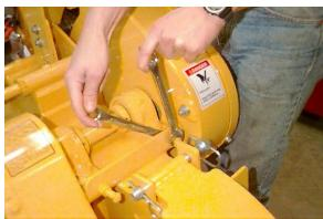
Replace Poly Chain® belt guard cover and bottom cover and tighten bolts.
