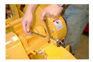
Remove the four bolts on the cutter wheel bearings. Cutter wheel will be free from machine at this point. With the Poly Chain® belt removed, you can start the machine and raise the boom up.
