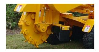
A locking pin is provided to hold cutter wheel in position during tooth removal and re-installation. Locking pin will only lock on outer teeth.
