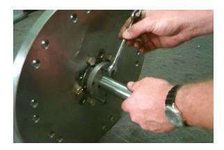
Place cutter wheel, bushing and bearings back on new shaft. Place back up under machine and lower boom box on to bearings.
