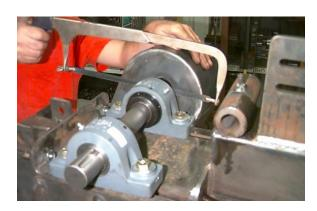
• Remove old bearings and shaft and replace with new bearings and shaft. Be sure to turn jackshaft with the longest keyway pocket toward the Poly Chain® belt side of the boom and make sure that the locking collars on the bearings are facing inward. Bolt new bearings and jackshaft back into place. Just snug bolts down, do not tighten all the way down, you will need to move them later to adjust belt tension.
