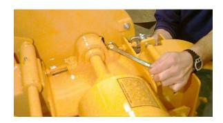
• Loosen the jam bolts in the back and move the bearings back.
