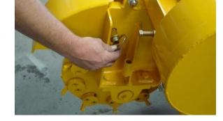
A Tooth Setting Gauge (P/N 0450111) is provided with each machine for proper tooth installation. Line all teeth up with the inside edge of the groove in the gauge. Set <u>ALL</u> teeth to this edge with gauge against pocket, not against cutter wheel.
