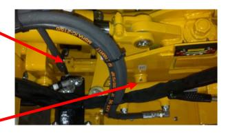
Grease bottom pivot bearings monthly. Use Texaco® Starplex II grease. You cannot over grease this area all parts are heattreated.
