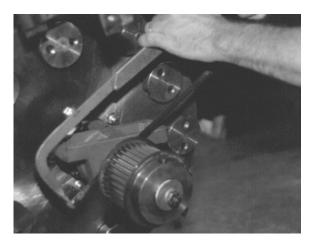
Remove Poly Chain® sprocket by removing the bolts inside the sprocket and tapered bushing. Then screw one bolt into third hole to push sprocket off tapered bushing to remove.
