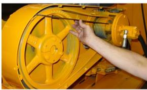
• There are two setscrews in each bearing. Tighten one of them down, remove one, and punch a start point in the shaft to drill a 5/16" diameter hole just deep enough for the screw to enter the shaft. Do this for all four setscrews. This will help prevent shaft from spinning inside of bearing. When replacing setscrews in bearings, use LocTite® 242 to prevent screws from loosening up.
