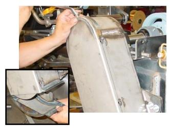
Remove Poly Chain® sprocket by removing the bolts inside the sprocket and tapered bushing. Then screw one bolt into third hole to push sprocket off tapered bushing to remove.
