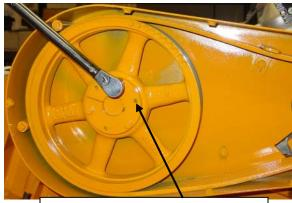
AFTER REMOVING BOLTS, SCREW BOLTS INTO THE THREADED HOLES TO PUSH THE BUSHING OUT OF THE PULLEY
