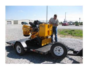
The model SP5014TRX can be loaded into a pick-up truck, but requires increased safety precautions against tipping. Tie-downs, a sturdy and stable loading ramp and extra caution are required.
