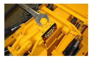
If the main pivot bearings need replacing, you will have to remove the top pin and slide the main pivot out and install the new bearings. **See Upper Pivot Assembly for breakdown.**
