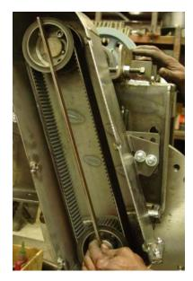
After replacing the jackshaft pulley and bushing, use a straight edge and align the jackshaft pulley with the engine pulley.
