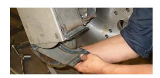
Grease boom pivot monthly, swing cutter wheel to the right to access grease fitting.
