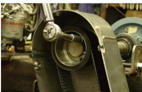
• You may cut the jackshaft between the bearings and the Poly Chain® guard.
