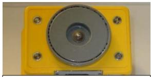
REMOVE THE BACK COVER TO ACCESS THE BATTERIES – THERE ARE 4 SCREWS HOLDING IT IN PLACE. THE BATTERY COMPARTMENT IS LABELED FOR CORRECT BATTERY ORIENTATION.
