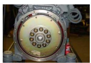
When parts have been removed, clean the engine flywheel with a cleaning solvent and check for burrs around the holes and on the surface of the flywheel. Use a very fine sand paper to remove any burrs.
