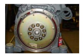
Put anti-seize (coupling lubricant) on the inside of the coupling. Line up external splines with the coupling ID and slide the stub shaft plate into place.
