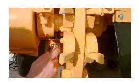
• Check setscrews in jackshaft bearing collars and in boom bearing collars for tightness weekly.
