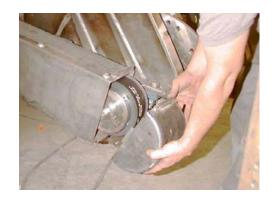
• Check cutter wheel, pockets, and teeth for wear daily. If any repair is needed, see Servicing Cutter Wheel section for further instruction.
