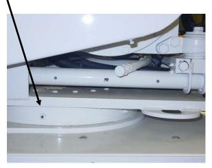
Also when greasing bearing, inspect seals, making certain that they are in proper position in grooves and intact. Check tightness of mounting bolts and retighten if needed. Be alert to changes in rotation, unusual sounds, and vibrations.
