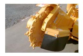
• Check setscrews in cutter wheel bearing collars for tightness weekly.
