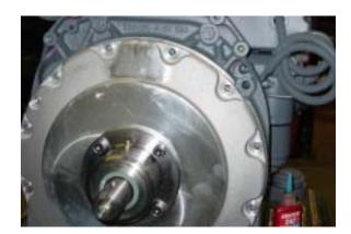
• There are two threaded holes that can be used to push the shaft plate off the engine mount. Insert two of the bolts that were removed from the stub shaft plate and slowly screw them in until the plate breaks loose. Leaving a couple of bolts screwed in slightly may help to keep the assembly from dropping when separated from the engine.
