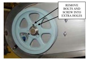
Remove the bolts holding the belt guard onto the machine and remove the belt guard.
