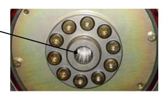
Make sure the grease fitting is on the top of the assembly. Replace the 10MM-1.5 x 30MM bolts and torque to 35 ft. lbs. There are eleven bolts holding the plate to the engine.
