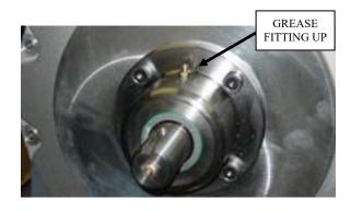
• Remove the grease fitting and replace with the grease fitting extension supplied with the machine.
