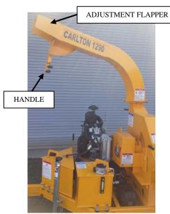
• There is an adjustable flap on the end of the discharge chute. This flap is adjustable in the vertical direction to help control the height and distance of the chips being discharged. To adjust this flap pull down on the handle and rotate the flap up or down to desired position.
