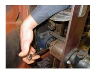
• Replace the rubber guard and bolt into place using the two 3/8" bolts that were removed. Tighten the bolts.
