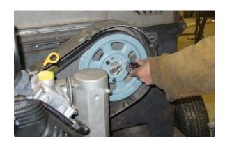
• Go to REPLACING ENGINE BELT section to replace belt and adjust tension.
