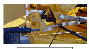
LOOSEN THE JAM NUT AND ADJUST THE SLIDE LOCK HANDLE
