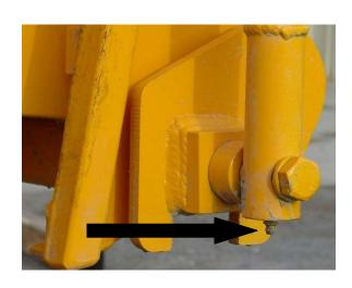
• Apply a light coating of oil to the feed control linkage **weekly**.
