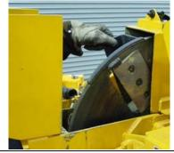
ROTATE CUTTER DISK TO CHECK FOR BINDING
