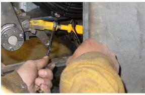
HOLD JAM NUT WITH ONE WRENCH AND ADJUST CLEVIS USING ANOTHER WRENCH. TURN COUNTER-CLOCKWISE TO TIGHTEN BELT TENSION AND CLOCKWISE TO LOOSEN BELT TENSION.
