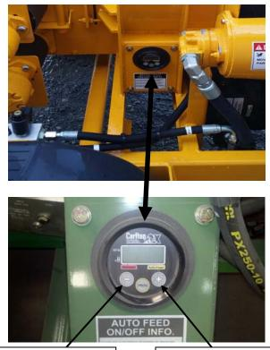
AUTO-FEED OFF (PRESS AND HOLD FOR 2 SECONDS TO TURN OFF)
