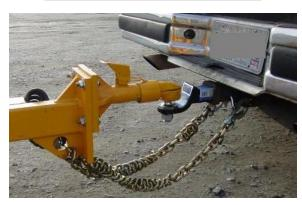
• Connect chipper lights to the tow vehicle. Observe light operation to insure correct electrical connections.
