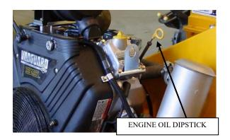
Check and maintain proper engine oil, fuel tank, and hydraulic oil tank levels. Make sure engine is cool before checking.
