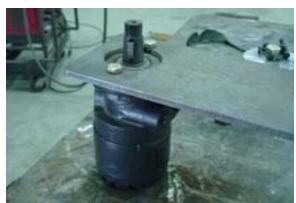
• Replace with new motor. Clean the threads on the motor, the 1" nut, and the coupling with degreaser before beginning to replace all the parts.
