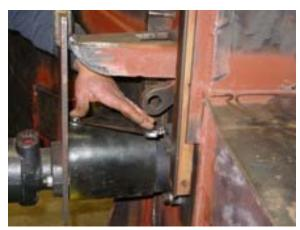
• Remove the three bolts (3/8") from the bushing and screw these bolts back into the three threaded holes in the bushing to push the motor assembly off the bushing. Screw these bolts in a little at a time to take the assembly off without applying more pressure to one side than the other.
