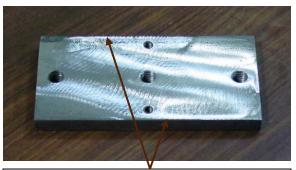
THE ANVIL HAS FOUR WORKING EDGES. TWO OF THESE EDGES ARE SHOWN ABOVE. FLIP THE ANVIL OVER FOR THE OTHER TWO EDGES.
