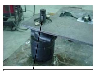
LINE UP KEY WITH KEYWAY ON COUPLING
