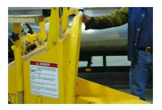
ALWAYS VERIFY CORRECT FUNCTION OF THE FEED CONTROL BAR BEFORE CHIPPING ANY MATERIAL.
