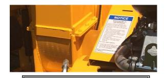
DANGER: Do not open the cutter disk hood until the cutter disk has come to a complete stop. Do not perform service on the cutter disk or knives without installing the disk lock pin.
