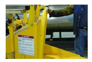
Push the throttle over into the low position so that the engine can slow down (idle) and the cutter disk can be disengaged.
