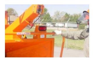
Push the throttle arrow down to an idle so that the engine can slow down and the clutch can be disengaged.
