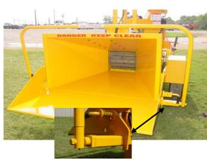
• Apply a light coating of oil to the feed control linkage weekly.
