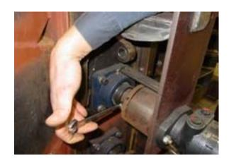
Reconnect the hydraulic hoses making sure to connect them in the right order, see markings made when hoses were removed. If hoses are reversed, the feed wheels will work in reverse. Change hoses if this happens to make feed wheels turn correctly.
