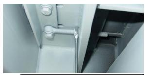
TIGHTEN THE INSIDE NUTS TO SHORTEN THE CLEARANCE BETWEEN THE KNIFE AND ANVIL
