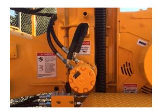
• Replace the rubber guard and bolt into place using the two bolts that were removed. Tighten the bolts.
