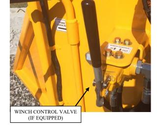
7. Pull the tree to the chipper using the winch control valve.
