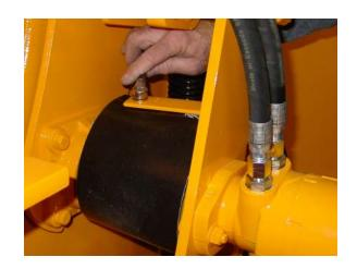
Before changing the feed wheel motor, release the hydraulic pressure. Mark the location of each hose, possibly with an R and L for right and left hoses. Then disconnect the hydraulic hoses and cap the ends of hoses and the connections on the motor.
