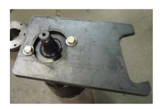
• Put the coupling onto the motor and line up key and keyway – always use new key. Use a rubber mallet to seat the coupling. Strike the coupling a couple of times. Apply LocTite 262 (red) to the 1" nut and screw in place. Torque the nut to 150 ft. lbs. Strike the coupler again a couple of times with the rubber mallet to finish seating and torque the nut to 150 ft. lbs. again.
