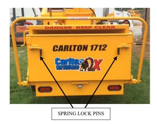
• Secure the discharge chute. Rotate the discharge chute back over the chipper and lock the swivel releasing the lock pin into one of the lock grooves. Make sure the height adjustment is at the lowest position so that the chute will not be high enough to hit any overhead obstructions and secure the handle. The flap on the end of the discharge chute needs to be lowered as far as possible so that no debris comes out during travel.
