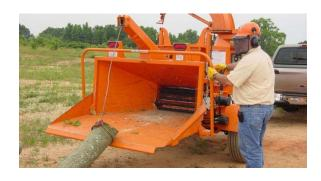
9. When the tree is in the infeed chute, remove the winch rope. Rotate the winch selector valve back to the left (clockwise) and follow the standard operating procedures for chipping the material.
