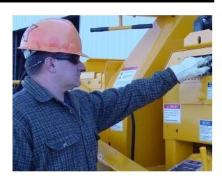
BECAUSE OF MACHINE VIBRATION, ALL EQUIPMENT ATTACHED USING SCREWS OR BOLTS AND NUTS SHOULD BE CHECKED REGULARLY FOR TIGHTNESS. ALL SCREWS, BOLTS, AND NUTS NEED TO BE INSPECTED FOR TIGHTNESS AND WEAR. ALL SCREWS, BOLTS, AND NUTS THAT WON'T STAY TIGHTENED OR THAT HAVE WORN, CHIPPED, OR MISSING THREADS SHOULD BE REPLACED.
