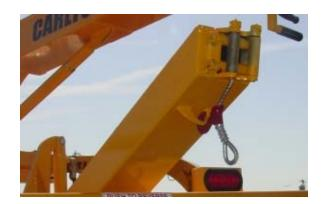
When a tree is too large to carry to the chipper, use the winch to pull the tree into the infeed chute.
