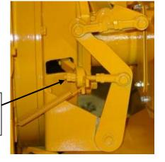
ADJUSTMENTS SHOULD BE MADE USING THESE TWO HEX NUTS
