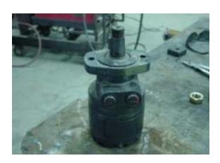
• Attach the torque arm to the new motor using the 1/2" bolts that were removed. Tighten the bolts and torque to 120 ft. lbs.
