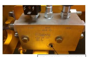
REMOVE PLUG AND INSTALL PRESSURE GAUGE
