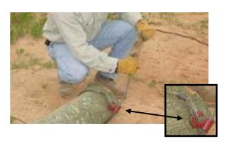
6. Lock the winch drum freewheel selector back into drive position. Once the winch rope is attached to the material to be winched to the chipper, pull the freewheel bar back up engaging the winch drive motor to the winch drum
