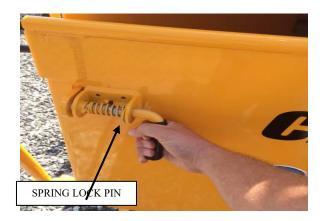
During transportation the infeed tray will be closed and locked using the spring lock pins attached. At the job site, release the lock pins and lower the tray.
