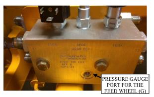
Adjust pressure only if necessary and after testing with a pressure gage. To increase pressure turn clockwise until it bottoms out. Recheck pressure. Contact J. P. Carlton or your dealer for more information.
