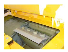
• Cutter drum must rotate freely. This will help insure there are no foreign objects inside the cutting chamber and there is ample knife to anvil clearance. (The cutter drum lock pin will have to be pulled out of cutter drum to check rotation. Replace pin after checking rotation to perform further inspections.)
