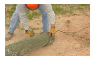
5. Secure the winch rope through the loop never on the rope itself.
