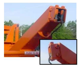
• Grease winch drum every 30-40 hours of operation as necessary. Use only Texaco® Starplex II grease.
