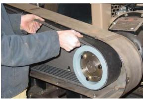
• Remove bolts from the bushing and screw each bolt into the threaded holes to push sheave off bushing. Screw bolts in equally to prevent damaging the bushing or the sheave, especially if you plan to use either one again.
