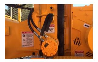
Remove the three bolts from the bushing and screw these bolts back into the three threaded holes in the bushing to push the motor assembly off the bushing. Screw these bolts in a little at a time to take the assembly off without applying more pressure to one side than the other.
