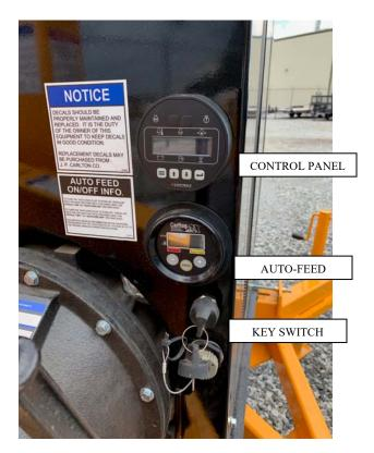
Throttle, tachometer, temperature gauge, and oil pressure gauge can be found on the control panel.
