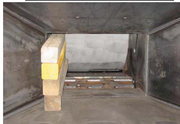
UPPER FEED WHEEL MUST BE RAISED, PINNED, AND BLOCKED
