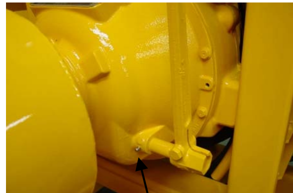
CROSS SHAFT & ENGAGEMENT LINKAGE
