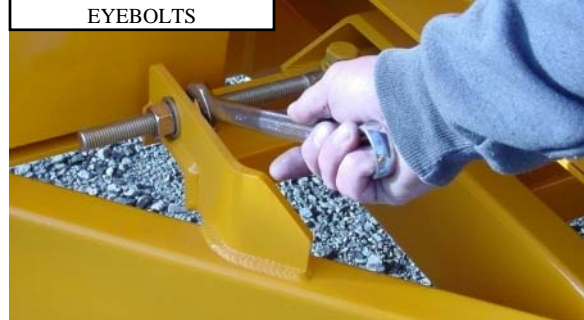
LOOSEN INSIDE JAM NUTS ON ADJUSTMENT EYEBOLTS
