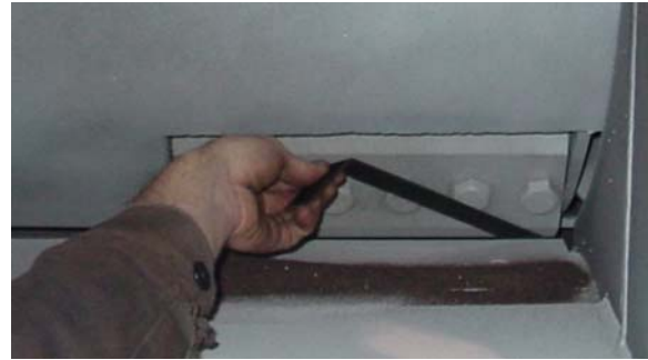
CHECKING CLEARANCE AT BOTTOM OF KNIFE ASSEMBLY
