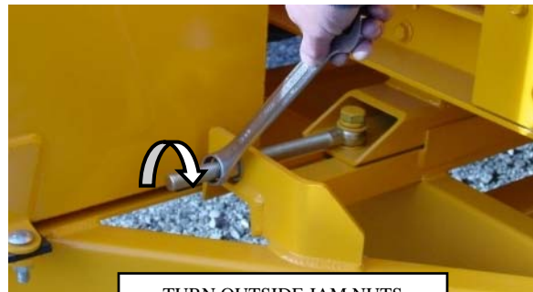
TURN OUTSIDE JAM NUTS CLOCKWISE TO TIGHTEN BELT
