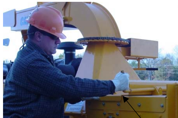
NO GAPS OR OPENINGS AROUND DOOR
