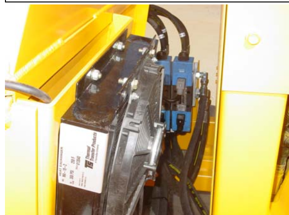
THE OIL COOLER ON THE 15" DRUM CHIPPER IS LOCATED BESIDE THE ENGINE AS SHOWN HERE
